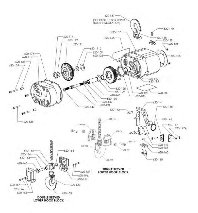
MODEL SLA AIR HOIST MECHANICAL PARTS EXPLODED VIEW
