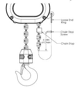
Figure 12. Attaching Loose End of Chain
